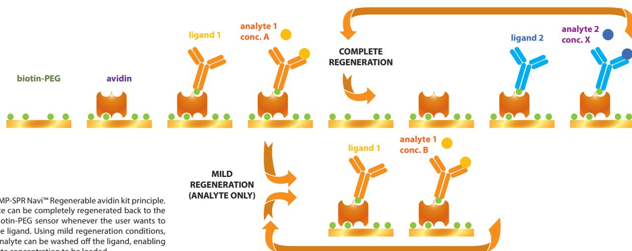
**Figure 1.** MP-SPR Navi™ Regenerable avidin kit principle. The surface can be completely regenerated back to the original biotin-PEG sensor whenever the user wants to change the ligand. Using mild regeneration conditions, only the analyte can be washed off the ligand, enabling next analyte concentration to be loaded.
