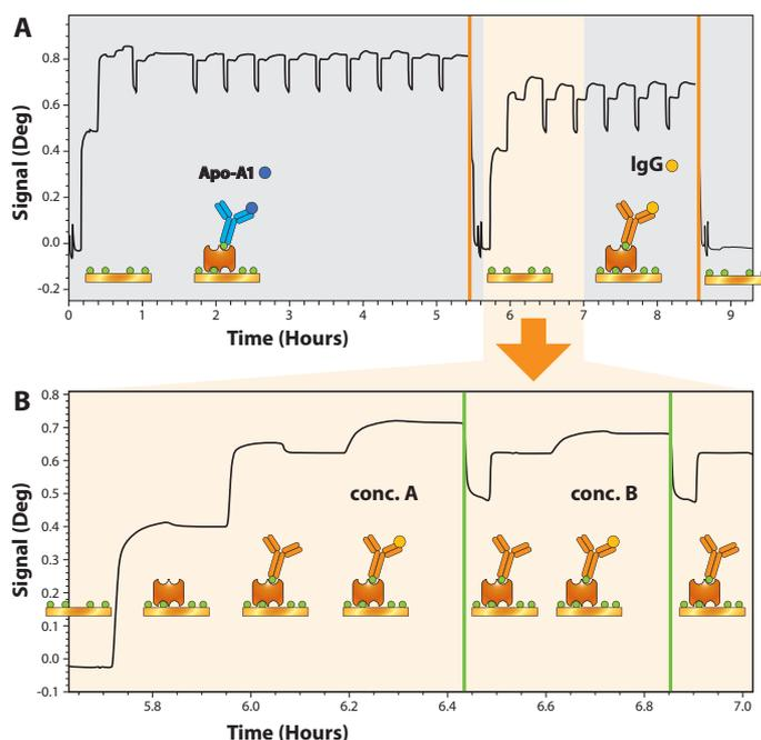
**Figure 2.** Measurement sensogram representing raw data of IgG and Apo-A1 concentration studies with MP-SPR Navi™ Regenerable avidin kit. A. Full measurement sensogram. Orange lines represent the time points of complete regeneration B. Close-up represents anti-IgG immobilization with biotin-avidin bridge and measuring the first two analyte concentrations. Green lines represents the time points of mild regeneration.
